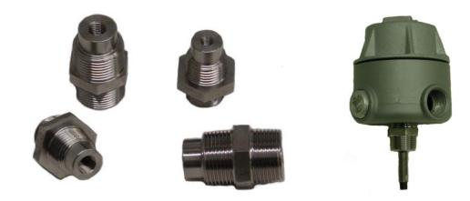
CMCP offers the CMCP-4190 for probe installations where the shaft is only a short distance from the bearing housing. The probe adapter is a 1/2" or 3/4" NPT threaded on either end for mounting to the housing, and a conduit head. The CMCP4190 is manufactured from Stainless Steel. The ID thread is available to fit the 2 common eddy probe thread sizes. For particularly long probes an optional deep conduit head is available.
